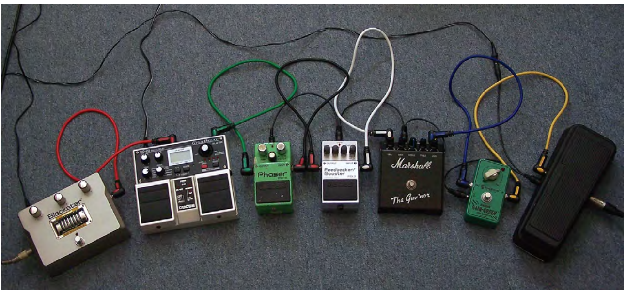
Fig. 1 A chain of stompboxes – note that the signal path runs from right to left, as the input on most pedals is on the right hand side and the output is on the left.
